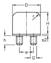
$$\begin{array}{lll} D & = 125 \\ e & = 63 \\ G & = M16 \\ H & = 100 \\ h & = 36 \\ Load capacity F (kN) = 150.0 \\ Load capacity f (mm) = 55 \\ Load capacity W (J) & = 2240 \\ \end{array}$$
